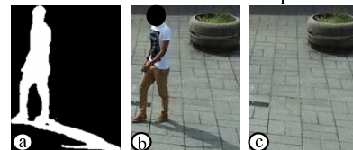
Figure 3: Outputs of background subtraction: foreground mask (a), foreground image (b) and mean background image (c).
