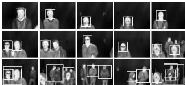
Figure 2: Examples of the detection using Haar Cascade algorithm with the improved classifier for thermal images.
