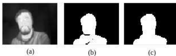
Figure 1: In (b) the segmentation of the thermal image (a). The result of applying the morphological operation is presented in (c).
